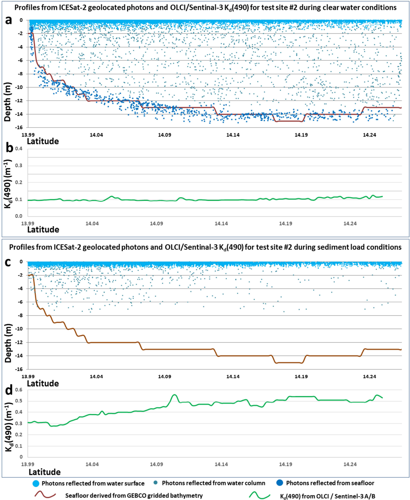
Figure 5. Bathymetric profile from ICESat-2 geolocated photons and corresponding profile of K_d(490) derived from level-2 OLCI of Sentinel-3 A/B mission for the extent containing shallow coastal waters at the eastern part of Nellore city, Andhra Pradesh, India. The ICESat-2 and Sentinel-3 acquisition overlap is \pm 24 hours. (a) Bathymetric profile during clear water conditions with an overlay of the surface profile from GEBCO gridded bathymetric data. (b) Profile generated from the K_d(490) layer for the same extent as shown in (a). (c) Bathymetric profile during sediment accumulation period with an overlay of the surface profile from GEBCO gridded bathymetric data. (d) Profile generated from the K_d(490) layer for the same extent as shown in (c).
